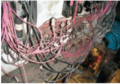
Control panel in a overhead bridge crane.
