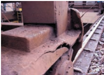
Stell structure damages caused by wery rough handling.
