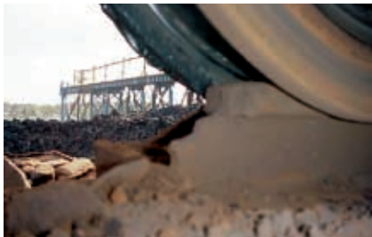
Bridge wheels badly worn, rail broken, no brakes etc.
